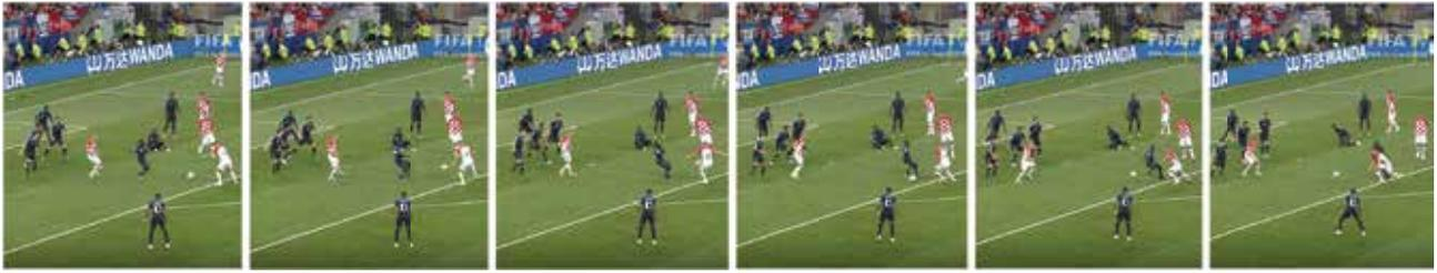
Example of a live video stream: Inter-Frame Compression can take advantage of the minimal differences between frames to obtain very high compression but must buffer multiple images to be effective.
