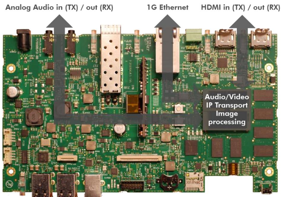
Figure 2 - Viper hardware board with HDMI, analog audio and Ethernet interfaces.
