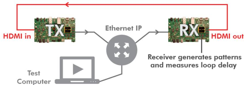
Figure 3 – Test setup used for the latency measurements.
