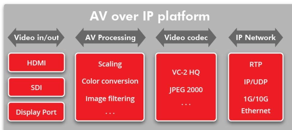
Figure 1 – Block diagram of the architecture of a typical AV over IP transmitter or receiver
